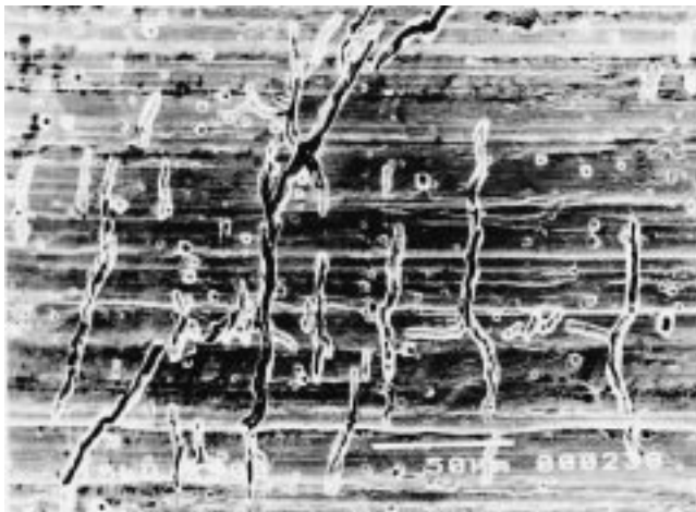
Fig. 5 SCC of ground state after immersion in MgCl_2 solution at 40 g/L heated at 140 °C
